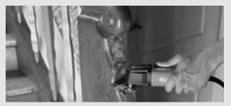
Six replaceable profiles of the profile sanding set enable you to sand cramped spaces, in grooves and on profiles – completely comfortable and with 300% improvement in sanding capacity. The flexible hollow sections perfectly adapt to various conditions.
