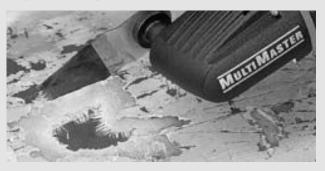
E-Cut saw blades for universal application with wood, fibre-glass-reinforced plastic and many other plastics. High cutting speed. Ideal for use on fitted parts. No free space required alongside or behind the work piece.
