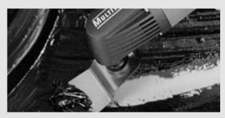
The rigid stopping knife can be used to remove underseal, residual carpet and tile glue, scale, damaged coatings, etc.
