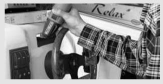
For sawing tasks in places that are not easily accessible, or for small grooves. Cutouts from as little as 10 mm wide. Exceptionally suitable for all sharpening tasks, in combination with the diamond file and the 15° clamping plate.
