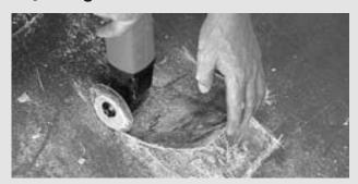
The HSS saw blades help you to saw fibreglass, carbon fibre-reinforced plastic, wood and sheet metal up to 1 mm.
