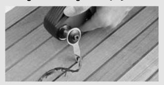
The cutter blade ideal for rapid and secure cutting out of panelled deck sealing materials is also suitable for problem areas such as cabins, rails, gunwales, cleats and curves.
