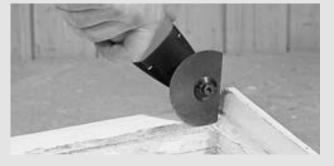
Use the saw blades to remove putty from single and multi-layered glazing without the risk of glass breakages and without laborious preparatory work.
