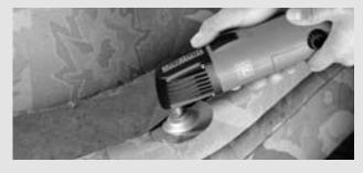
Ideal for upholsterers: sawing off and removing metal clamps with the cropped HSS saw blade.
