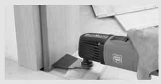
Grooves, cutouts and adapting parquet, laminate, fitted door jambs and skirting boards are easily achieved with the cropped E-Cut saw blades. The cropped saw blades enable you to work flush to the surface. The special toothing permits a superior cutting speed.
