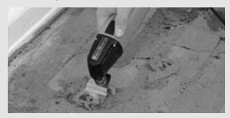
Residual carpet and tile adhesive, scale, underseal and damaged coatings are easily removed with the rigid stopping knife.
