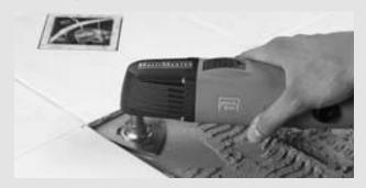
The carbide rasp produces optimum results when sanding down tile adhesive, sanding edges of tiles, coarse sanding wood, filler, paint and much more.
