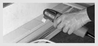
For sawing wood, putty and soft materials. HSS saw blades also for fibreglass, carbon fibre-reinforced plastic and sheet metal up to 1 mm. Cropped saw blades enable you to work flush to the surface. The segment blades allow you to cut at right angles without overcutting.
