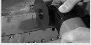
Use the HSS saw blade for sawing sheet metal up to 1.0 mm, wood, putty, carbon fibre and fibre-reinforced plastic. Cropped saw blades enable you to work flush to the surface. The segment blades allow you to cut at right angles
