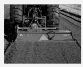
Adjustable offset allows the tiller to be used in a central or side position (pictured) with respect to the tractor's wheel track allowing you to till closer to existing plants and into deep corners. The chain-supported tailgate is self-leveling.
