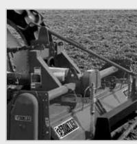
On the RT22 and RT23 Series, the hand cranks (or optional hydraulic kit) make adjusting the roller easy. Use a lower setting for more firming action, ideal for controlling wind erosion.
