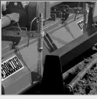
On the RT22 and RT23 Series, double springs provide consistent down pressure on the tailgate to level the tilled soil. Adjusting the height of the tailgate is easy: just remove the bolts and raise the tailgate to one of five settings. Use the low setting for a more level finish.
