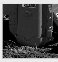
Heavy-duty wear shields on the RT23 Series help protect the gearcase from abrasion and premature wear.
