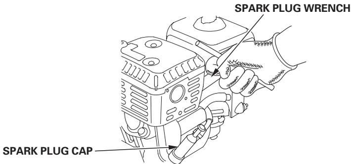
3. Inspect the spark plug. Replace it if the electrodes are worn, or if the insulator is cracked or chipped.
