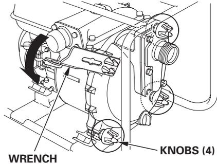
3. Remove the pump cover and the volute case from the pump casing, and remove any debris from pump casing and volute case.
