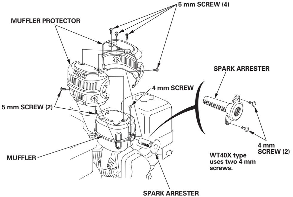
3. Use a brush to remove carbon deposits from the spark arrester screen. Be careful to avoid damaging the screen.
