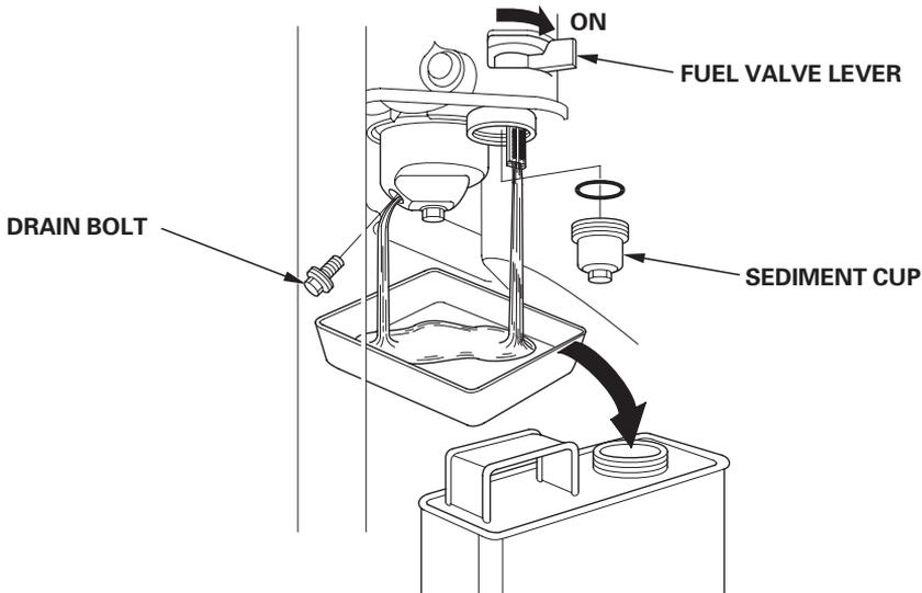
3. After all the fuel has drained into the container, reinstall the drain bolt and sediment cup. Tighten them securely.
