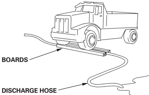
Driving over a discharge hose while the pump is running, or even possibly when the pump is stopped, may cause pump case failure.
